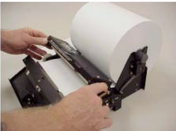
Figure 9 - GPT-1578 Top view with Cutter and Print Mechanism open
