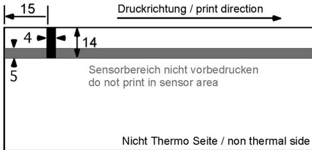
Control black marks must be printed using infrared absorbing color in the range of 910-950 nm. Optical density should be a minimum of 1.0.
