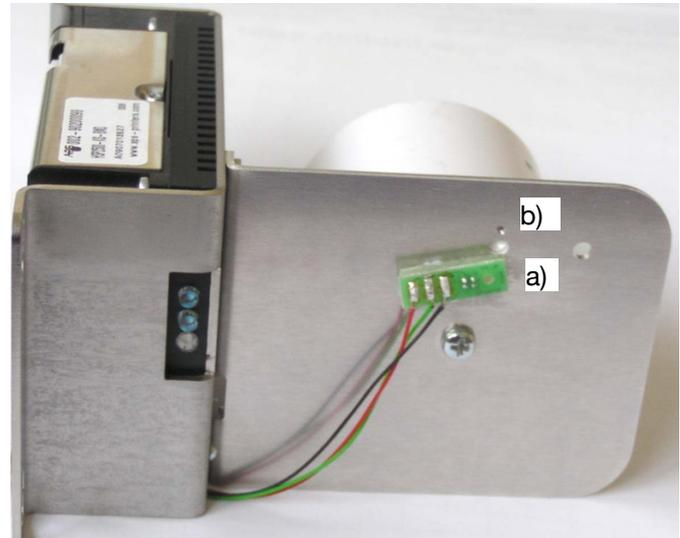
The sensor is plugged on the board.
