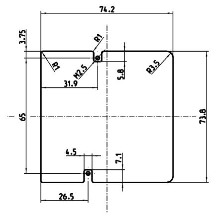
Partial installation in a plastic casing
