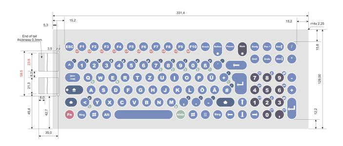
Matrix Configuration of the GFT-104 (Deviations in US Layout in red )
