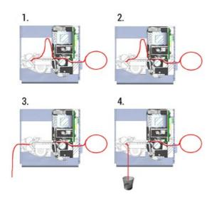
The loop-presenter (1.) transports the already printed paper, prior to Cut (2.) and paper output (3.), upward. Maximum paper thickness and ticket length need to be regarded, since loops can get to long and collapse or fall over and may cause a paper jam. Loop-Presenters can be offered with retract-function (4.).
