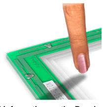
A finger is simulated by a silicon rubber plunger R8 (Round type 8mm size) hardness 60° at 200g at frequency 5Hz.
