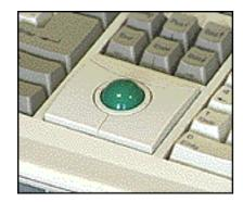
A <u>Trackball</u> which is compatible with Windows is integrated in the KTQ-95 keyboard. All functions of a mouse are offert to you without using important space on the desk. The practical trackball minimizes the movements of your for more comfort.
