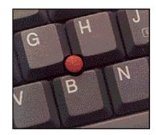
The Micro Joystick, known from application in laptops of IBM and Fujitsu, is very well suitable for the installation in keyboards and mice.
